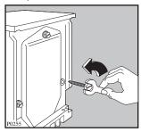
2. Remove the polystyrene base and take off the bottom panel by unscrewing the central screw..
